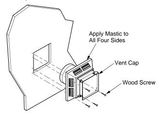
Figure 10 - Installing Horizontal Vent Cap
